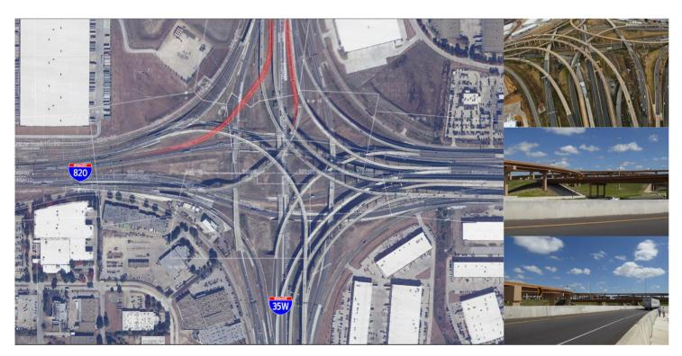
The works on the I820/IH 35W interchange include two new direct connectors in an already very structure-congested area that allow access to new Managed Lanes for traffic flowing from IH35 W to I820 WB and from I820 EB to I35W. Additionally, 9 minor bridges spanning over Mark IV Parkway and Little Fossil creek had to be replaced by new bridges with phased construction.
